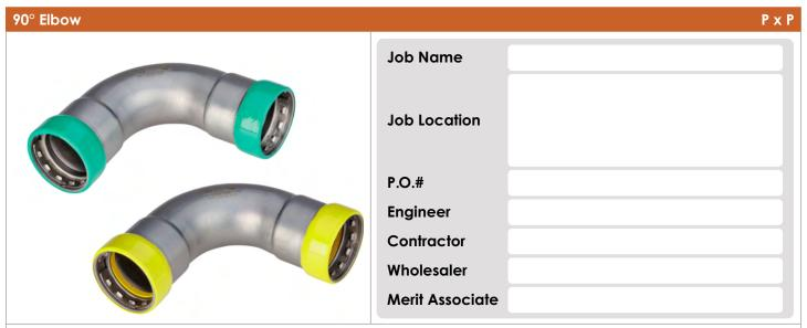
CarbonPress® 90° Elbow P x P is available in sizes 1/2" - 2" with an EPDM or HNBR sealing element.
