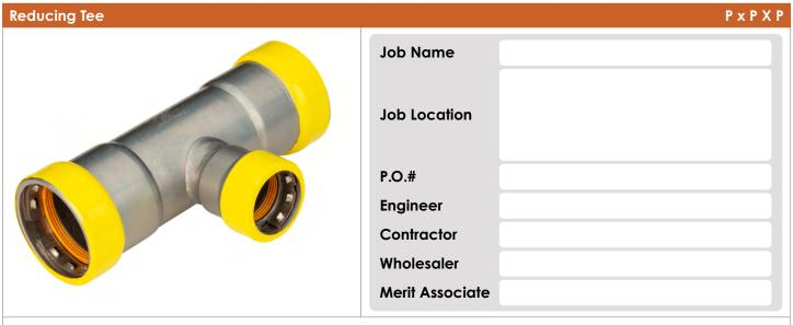
CarbonPress® Reducing Tee P x P x P is available in sizes 1/2" - 2" with an EPDM or HNBR sealing element.
