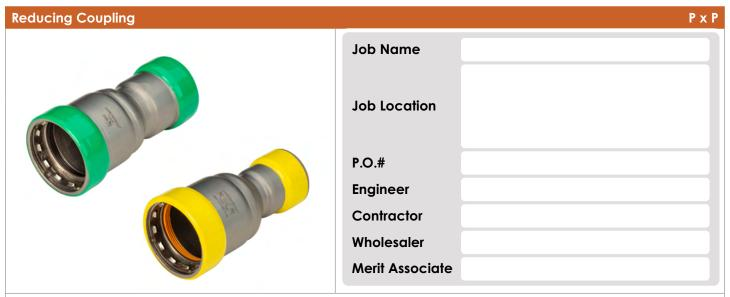
CarbonPress® Coupling Reducer P x P is available in sizes 1/2" - 2" with an EPDM or HNBR sealing element.
