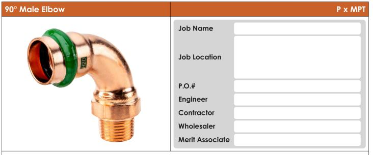
CopperPress® Small Diameter 90° Male Elbow P x MPT is available in sizes ½" x ½" - 2" x 2" MPT with an EPDM sealing element.
