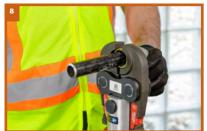
An incomplete press may reduce the pressure retention capabilities of the joint and lead to subsequent system leakage.
