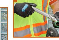
Once the jaw is removed from the fitting, the VIPR<sup>®</sup> will break off, indicating a complete press.
