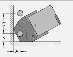
\*Loop-Type Jaw clearances. Dimensions may vary based on pressing tool. Refer to pressing tool manufacturer's instructions for specific dimensions. See page 26 for installation instructions.
