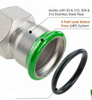
**Engineered sealing elements** are designed to leak before they are pressed, giving a visual indication of a connection that has not been pressed.
