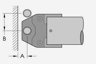
\*Loop-Type Jaw clearances. Dimensions may vary based on pressing tool. Refer to pressing tool manufacturer's instructions for specific dimensions. See page 26 for installation instructions.
