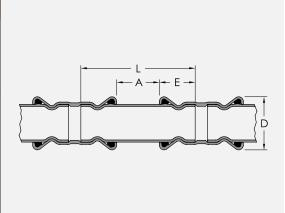
Minimum Fitting Distance is the recommended minimum distances between fittings to permit mechanical forming of the pipe during the pressing process.
