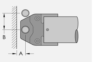
\*Loop-Type Jaw clearances. Dimensions may vary based on pressing tool. Refer to pressing tool manufacturer's instructions for specific dimensions. See page 13 for installation instructions.
