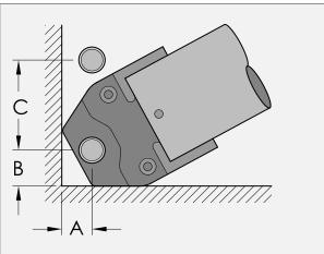
\*Loop-Type Jaw clearances. Dimensions may vary based on pressing tool. Refer to pressing tool manufacturer's instructions for specific dimensions. See page 13 for installation instructions.
